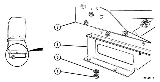
(3) Remove two nuts (4) and washers (5) from each side of seat frame (6).(4) Lift seat frame (6) off seat support (7).
