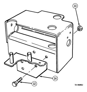
17-7. REAR CABLE TENSIONER REMOVAL/REPAIR/INSTALLATION (M984) (CONT).
