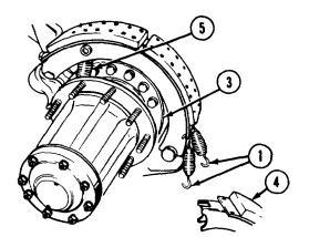
(5) Pry brakeshoes (2) away from cam (6) and install cam roller pins (7) and cam rollers (8).
