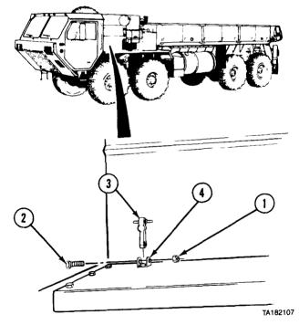
(1) Remove nut (1), screw (2), and holddown (3) from bracket (4).
