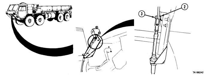
(2) Remove cotter pin (2) and clevis pin (3).
