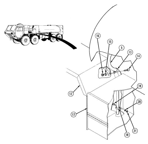
(5) Install vent hose (5) to fender (12) with clip (13), screw (14), lockwasher (15), and nut (16).
