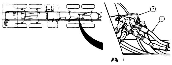
**NOTE** Tag and mark air lines and elbows before removal.
