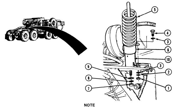
Some vehicles have a nut, lockwasher, washers, and a screw. Others have a flanged nut and screw.
