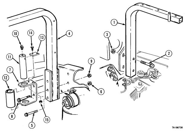
(1) Install right front fender support (1) with two screws (2) and nuts (3).
