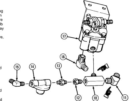
(6) Coat threads with pipe thread sealing compound and install four elbows (16) in bottom of brake relay valve (17).
