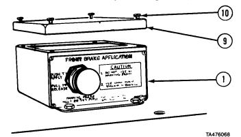
(6) Install cover (9) on box (1) and tighten four screws (10).
