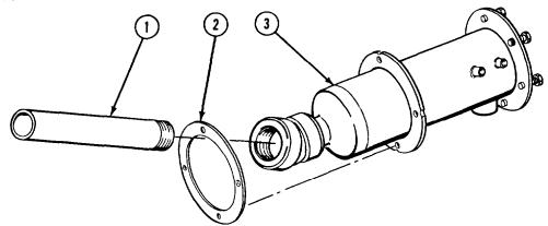
(1) Install pipe (1) and gasket (2) on filter housing (3).
