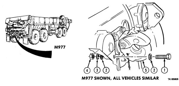
(1) Remove four screws (1), eight washers (2), four lockwashers (3), and four nuts (4). (2) Remove pintle hitch (5).
