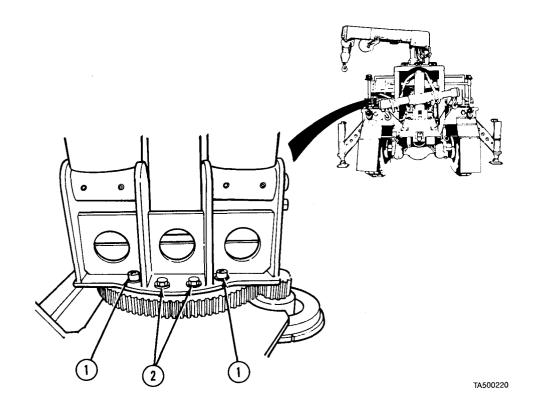
(1) Tighten two screws (1) and two screws (2) to 370 lb-ft (502 N·m).
