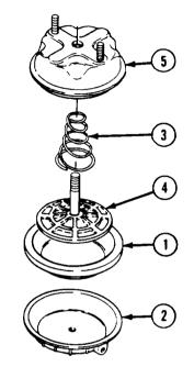
(4) Aline matchmarkers and clamp nonpressure housing (5) and pressure housing (2) together.
