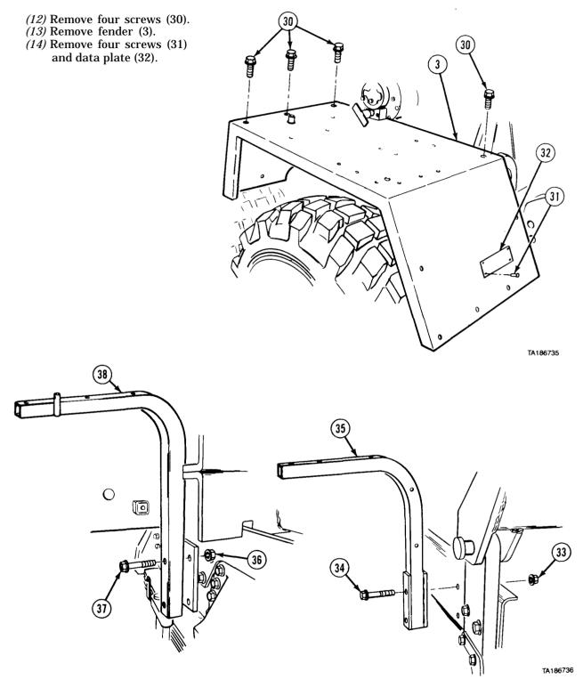
(15) Remove two nuts (33), screws (34), and left rear fender support (35). (16) Remove two nuts (36), screws (37), and left front fender support (38).
