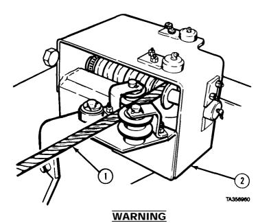
Always wear heavy gloves when handling winch cable. Never let cable run through hands. Frayed cable may cut hands severely.
