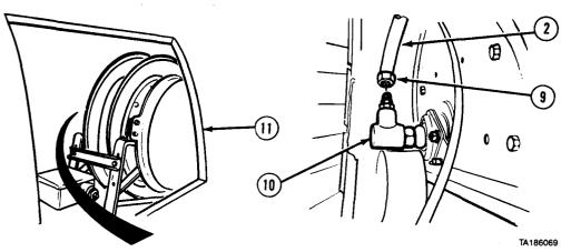
(5) Disconnect fitting (9) and remove hose (2) from swivel fitting (10).(6) Remove hose (2) from pump module (11).
