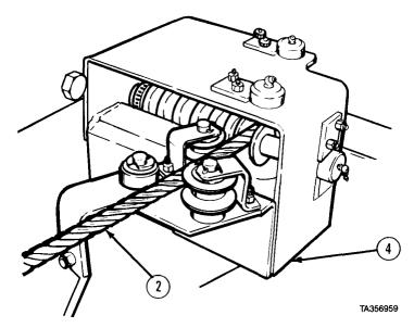
(3) Remove cable (2) from cable tensioner guide (4).
