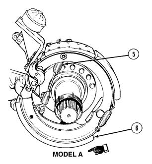
(2) Remove release spring (5) and let brakeshoe (6) drop down.
