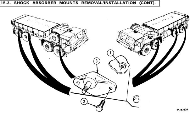
c. Shock Absorber Mounts Removal. Remove two nuts (1), screws (2) and shock absorber mount (3) from frame (4).
