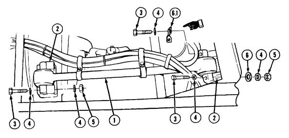
**NOTE** Do steps (1) through (7) for torque rods except torque rod No. 2 with front tandem crossmember/torque rod kit. Do steps (8) through (11) for torque rod No. 2 with kit.
