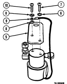
(5) Install mounting bracket (5), lockwasher (6), and screw (7).(6) Install lockwasher (8), ground wire (9), lockwasher (8), and screw (10).
