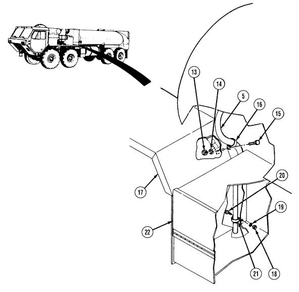
(5) Remove nut (13), lockwasher (14), screw (15), clip (16), and vent hose (5) from fender (17).
