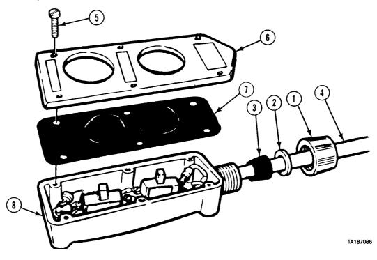
Loosen and slide cap (1), ring (2), and seal (3) down wire harness (4).
