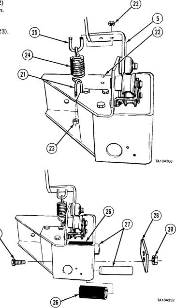
(11) Install two rollers (26) and two pins (27) with two lockplates (28), four screws (29), and locknuts (30).
