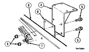
16-68. WRECKER BODY SUPPORTS (FRAME-MOUNTED) REMOVAL/INSTALLATION (M984E1).
