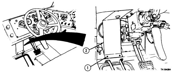
(1) Remove four screws (1) and remove light guard ('2).
