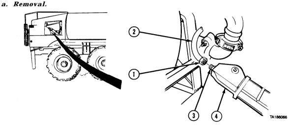
(1) Disconnect fitting (1) and remove hose (2) from fitting (3). (2) Remove fitting (3) from pneumatic actuator (4).
