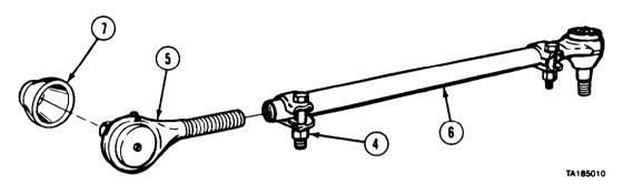
(2) Coat threads of drag link end (5) with antiseize compound.
