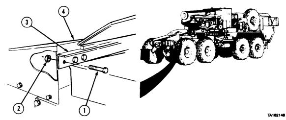
(1) Remove six screws (1) and nuts (2) to remove crosspiece (3) from fifth wheel ramp (4).
