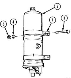
Brake and Air System Maintenance Instructions (Cont) 11-23. **AIR DRYER REMOVAL/INSTALLATION (CONT).** 13 12 7
