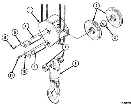
(1) Install hook block housing (1) on hoist cable (para 17-20).
