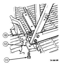
(5) Soldier A holds and removes two locknuts (10) while Soldier B removes two screws (11) and two mounting plates (12).
