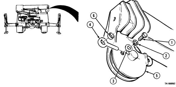
(1) Remove screw (1), lockwasher (2), washer (3), and pin (4) from boom (5). (2) Remove bushing (6) from pin (4).
