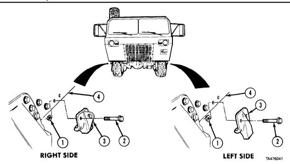
a. Axles No. 1 and No. 2 Axle Stop Removal. Remove two nuts (1), screws (2), and axle stop (3) from frame (4).
