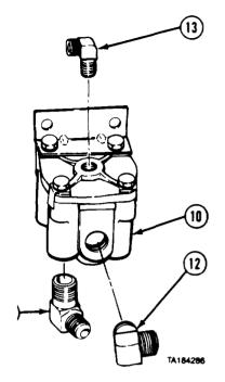
b. Front Brake Relay Valve Installation.
