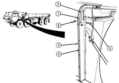
(1) Remove eight rivets (1) and rubber strip (2) from left side frame (3) and support (4).
