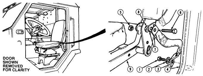
**NOTE** Both seat belts are removed the same way. Left seat is shown.
