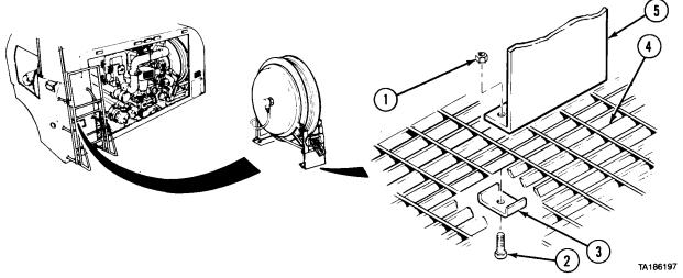
(1) Soldier A holds and removes two locknuts (1) while Soldier B removes two screws (2) and brackets (3) from grating (4) and hose reel (5).
