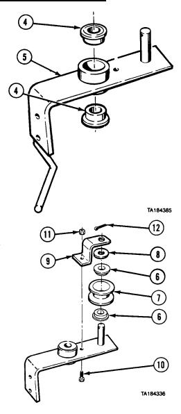
(3) Install two bearings (6) in roller (7).
