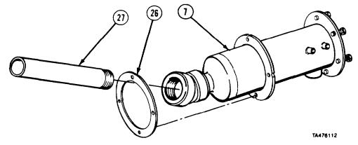
(10) Remove gasket (26) and pipe (27) from filter housing (7).
