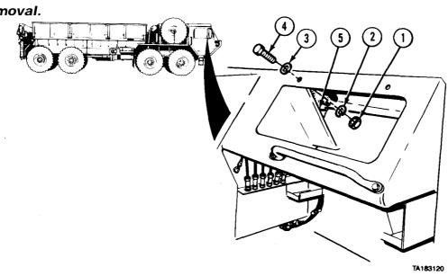
(1) Remove nut (1), lockwasher (2), washer (3), screw (4), and defroster hose guard (5).
