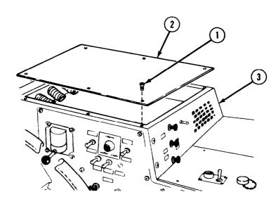
(1) Remove eight screws (1) and remove heater compartment cover (2) from heater control
