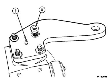
(5) Remove steering arm (4) from ball socket studs (10).
