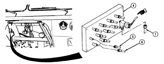
(2) Disconnect two air lines (5), eight air lines (6), and air line (7) from No. 4 air manifold (4).
