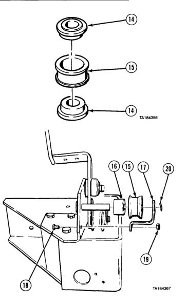
(7) Install spacer (16), roller (15), and S-bracket (17) with screw (18), nut (19), and cotter pin (20).
