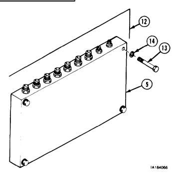
(6) Connect seven air lines (15), two air lines (16), and two air lines (17) on No. 4 air manifold (5).
