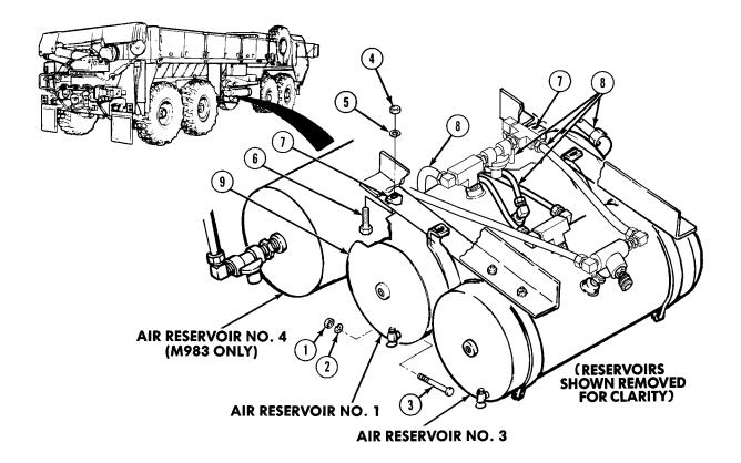
(1) Remove two nuts (1), lockwashers (2), and screws (3).
