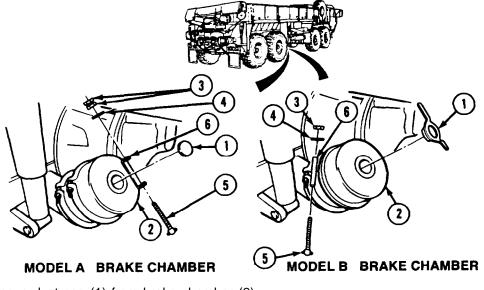
(1) Remove dust cap (1) from brake chamber (2).
