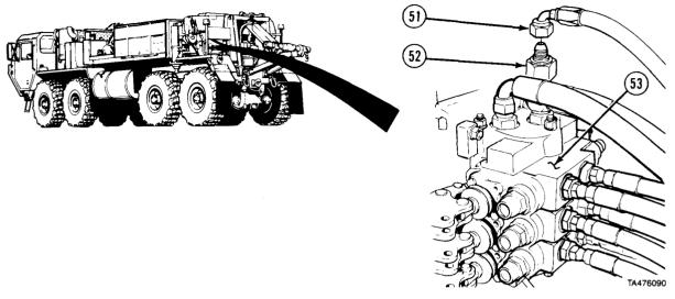
(18) Disconnect hose (51) from fitting (52) on retriever control (53).
