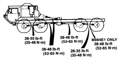
Figure 9-1. Capscrew Torque Limits
