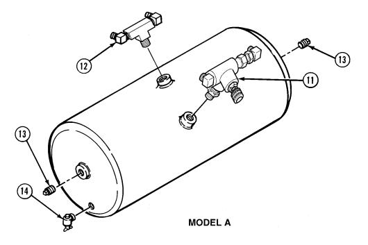
(5) Install four-way tee assembly (11), tee assembly (12), two plugs (13), and drain valve (14).
