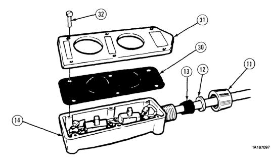
(18) Install gasket (30) and cover (31) on control box (14) with six screws (32). (19) Install seal (13), ring (12), and cap (11) in control box (14).
