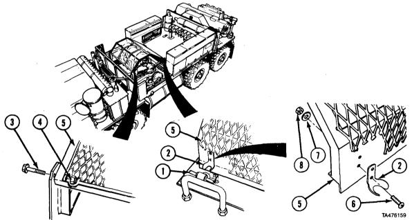
(1) Unhook two rubber hooks (1) from hook brackets (2).
