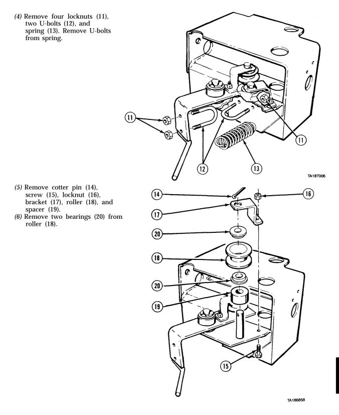
17-7. REAR CABLE TENSIONER REMOVAL/REPAIR/INSTALLATION (M984) (CONT).
