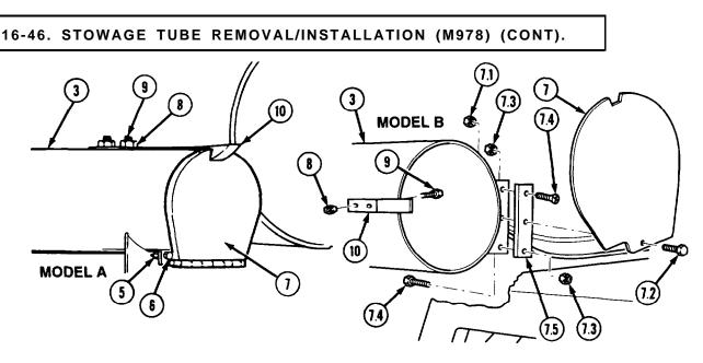
(2) Remove three nuts (5), screws (6), and tube cover (7) from stowage tube (3).
