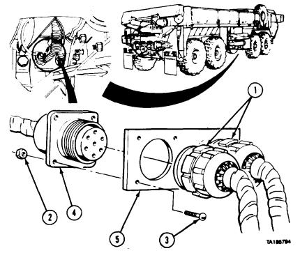
(1) Remove two connector plugs (1).(2) Remove eight nuts (2), screws (3), and two connector sockets (4) from bracket (6).
