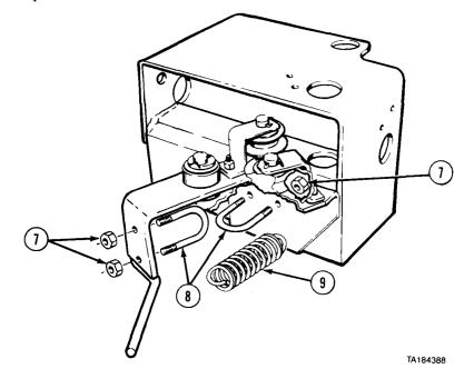
(4) Remove four locknuts (7), two U-bolts (8), and spring (9). Remove U-bolts from spring.
