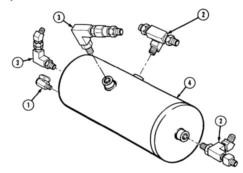
**NOTE** Tag and mark valves, fittings, and connectors before removal.
