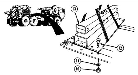
(5) Attach suitable lifting device and remove eight nuts (10), lockwashers (11), screws (12), and rear wrecker body support assembly (13).
