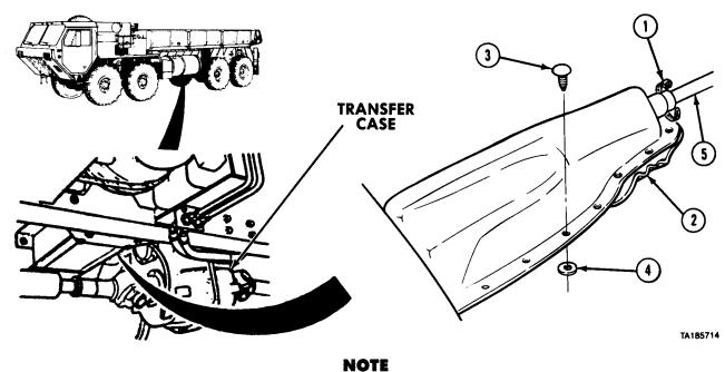
Boot is black plastic cover located on top right side of transfer case.
