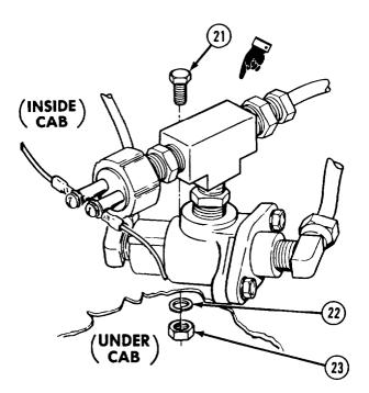
(10) Soldier A installs screw (21) while Soldier B installs lockwasher (22) and nut (23).
