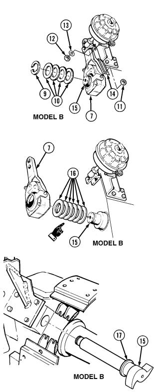
(6) Remove camshaft (15) and spacer (17).
