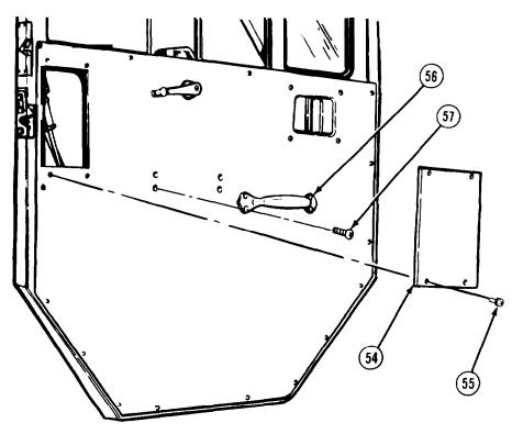
(37) Install cover plate (54) with four washer head screws (55), and lockwashers (58).(38) Install door handle (56) with four screws (57).
