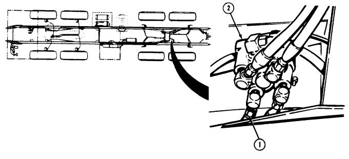
**NOTE** Tag and mark air lines and elbows before removal.
