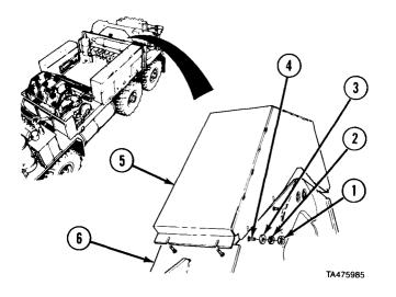
(1) Remove 12 nuts (1), lockwashers (2), and washers (3) from studs (4). (2) Remove outrigger cover (5) from outrigger beam assembly (6).
