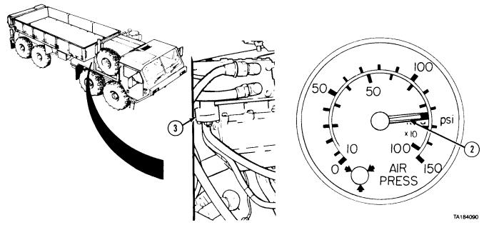
(3) After several minutes, gage needle (2) should stop at between 120 and 125 psi (827 and 862 kPa) as governor (3) cuts out. When governor cuts out, released air from air dryer can be heard.
