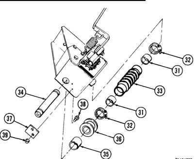
(15) Install three grease fittings (40) in pins (27 and 34).
