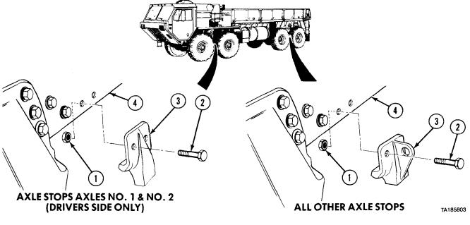
a. Removal. Remove two nuts (1) and screws (2) from axle stop (3) and frame (4).
