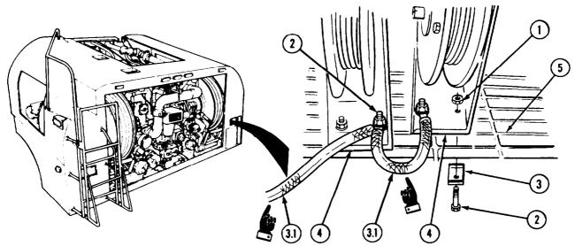
Both cable reels are removed the same way. Mark position of reels.
