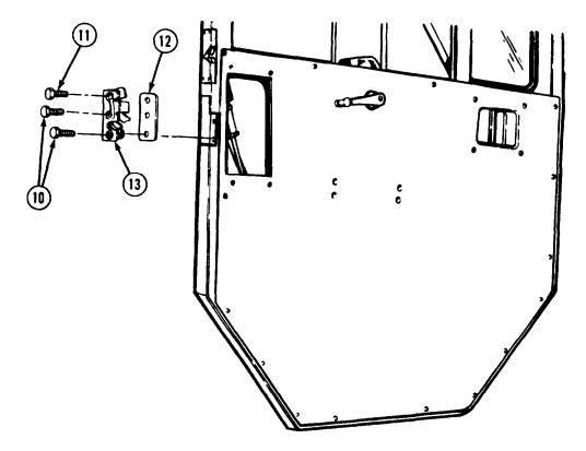
**NOTE** Latch must be in closed position to remove lock.
