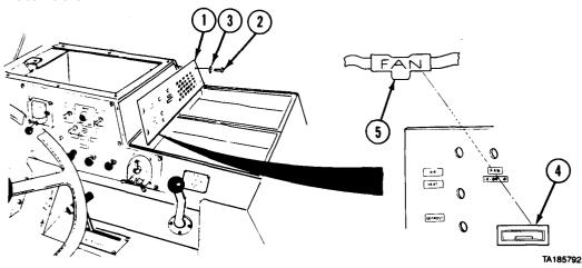
(1) Install center heater compartment cover (1) with four screws (2) and lockwashers (3). (2) Install five lenses (4).
