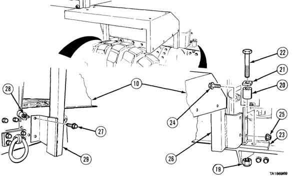
(7) Remove nut (19), spacer (20), washer (21), and screw (22) from crane mount (23).
