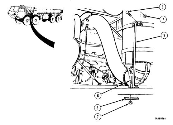
(2) Remove three screws (6), nuts (7), plate (8), and grab handle (9).
