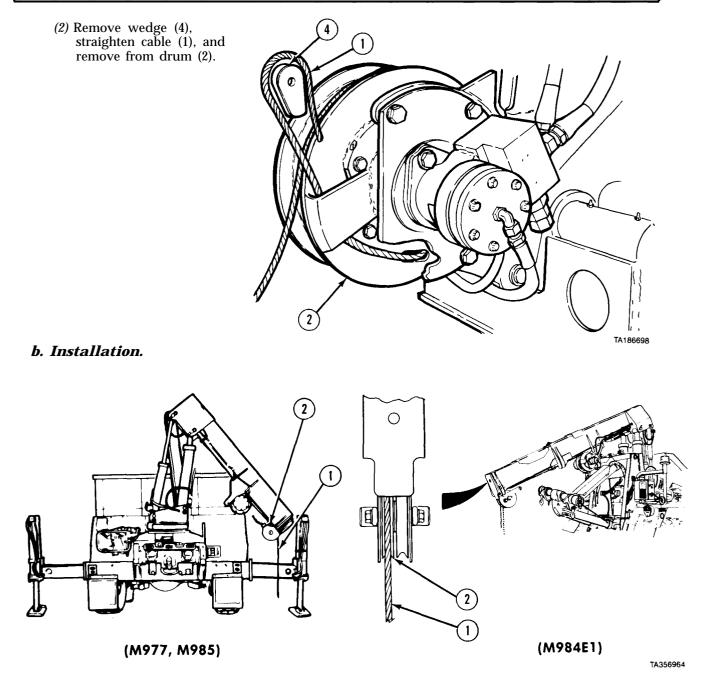
(1) Put cable (1) through boom sheave (2).
