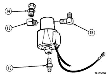
17-30. PTO SOLENOID REMOVAL/INSTALLATION (CONT).
