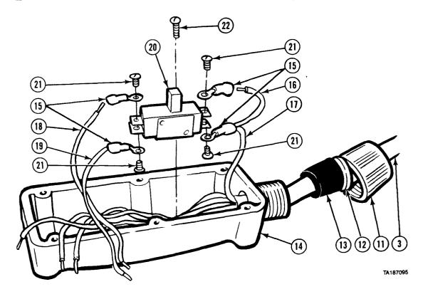
(8) Install cap (11), ring (12), and seal (13) on wire harness (3). (9) Install wire harness (3) in control box (14).
