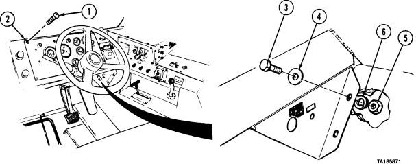
(1) Remove six screws (1) and move instrument panel (2) toward steering wheel.(2) Soldier A removes two screws (3) and washers (4) while Soldier B removes two nuts (5) and
