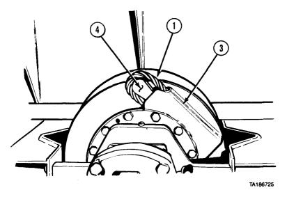
(2) Soldier A installs cable (1) in cable holder (3) while Soldier B installs cable anchor (4).
