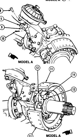
(7) Pry brakeshoes (11) away from cam (12) and install cam roller pins (13) and cam rollers (14).
