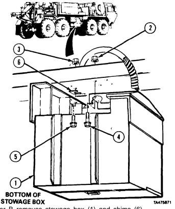
(4) Solder A operates lifting device while Soldier B removes stowage box (1) and shims (6).
