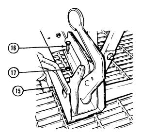
(7) Install bracket (15) with two screws (16) and locknuts (17).
