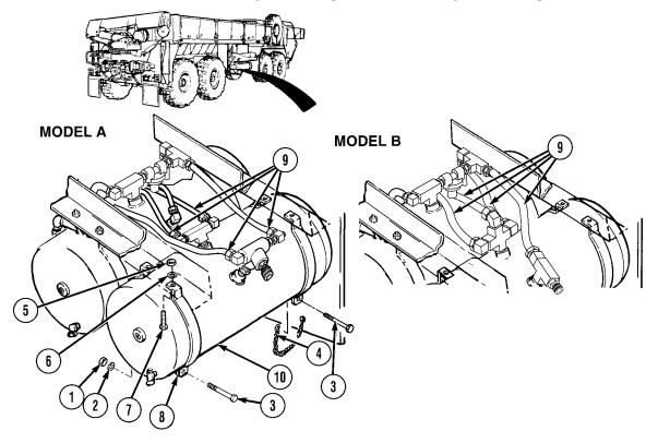
(1) Remove two nuts (1), lockwashers (2), screws (3), and one chain assembly (4).
