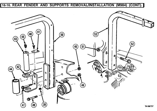
(17) Remove two locknuts (39), screws (40), and lockdate (41) from cable roller bracket (42),
