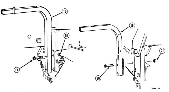
16-16. REAR FENDER AND SUPPORTS REMOVAL/INSTALLATION (M984) (CONT).
