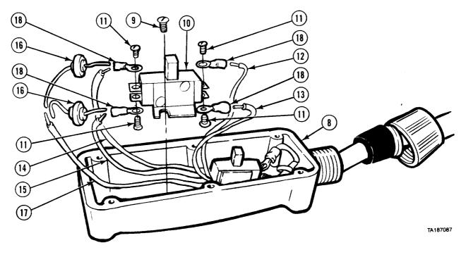
(3) Remove screw (9) and pull switch (10) from control box (8).
