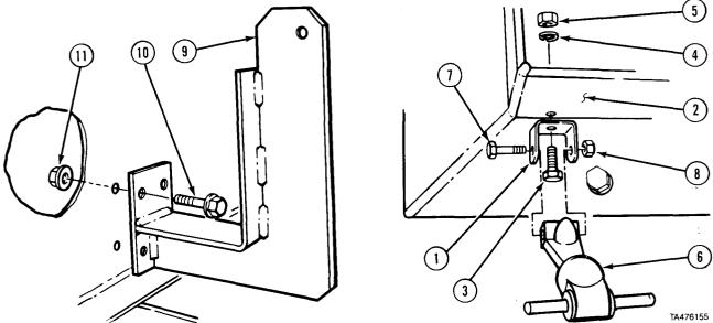
(1) Install two brackets (1) on frame (2) with screws (3), lockwashers (4), and nuts (5).
