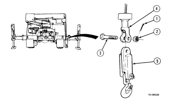
(1) Remove cotter pin (1), nut (2), and screw (3) from clevis (4). (2) Remove hook block (5) from clevis (4).
