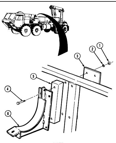
**NOTE** Both mounting brackets are removed and installed the same way.
