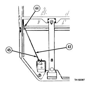
(27) If needed, adjust length of outer link rod (43) as follows:(a) Loosen jamnut (45).
