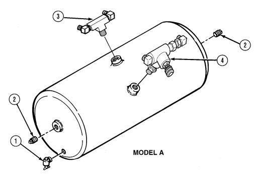
(1) Remove drain valve (1), two plugs (2), tee assembly (3), and four-way tee assembly (4).
