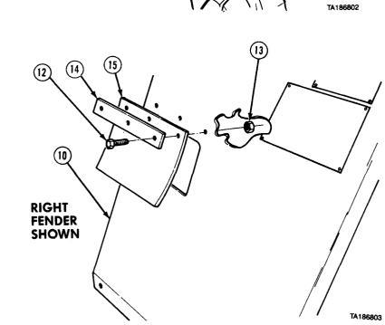
(3) Remove three screws (12), locknuts (13), holddown strap (14), and fender flap (15) from fender (10).
