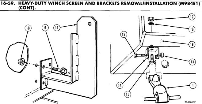
(4) Remove eight screws (9), nuts (10), and two brackets (11).
