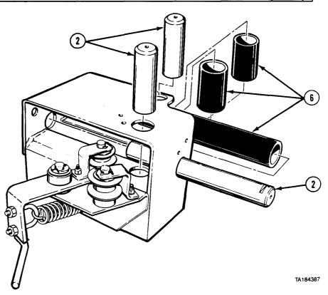
17-3. REAR CABLE TENSIONER REMOVAL/REPAIR/INSTALLATION (CONT).
