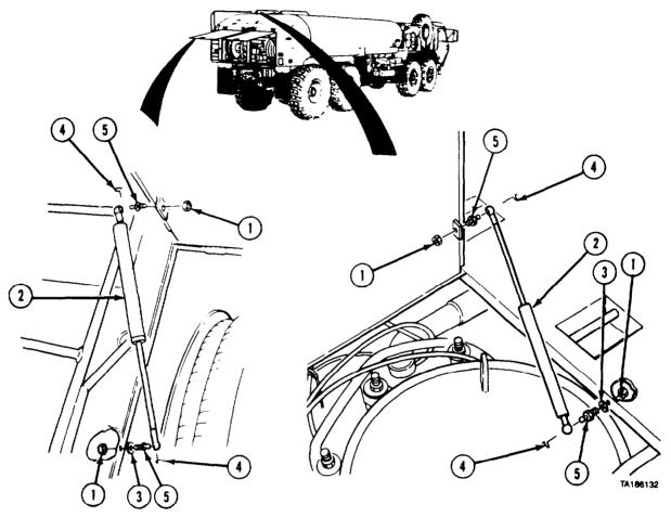
(1) Soldier A removes two locknuts (1). door piston (2). and washer (3) while Soldier B holds door.
