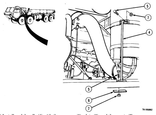
(2) Install grab handle (4) with three screws (5), plate (6), and three nuts (7).
