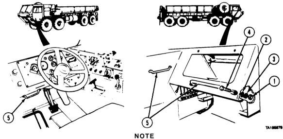
To remove any grab handle in or on cab, do step (1) only. To remove grab handle on air cleaner, do step (2) only. To remove grab handle on tire carrier and cargo box, do step (3) only.
