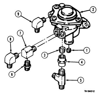
(4) Coat threads with pipe thread sealing compound and install elbows (7, 8, and 9) in spring brake control valve (2).
