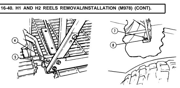
(6) Tighten two screws (4 and 7) and locknuts (5 and 8) to 15 to 25 lb-ft (20.34 to 33.89 N•m).
