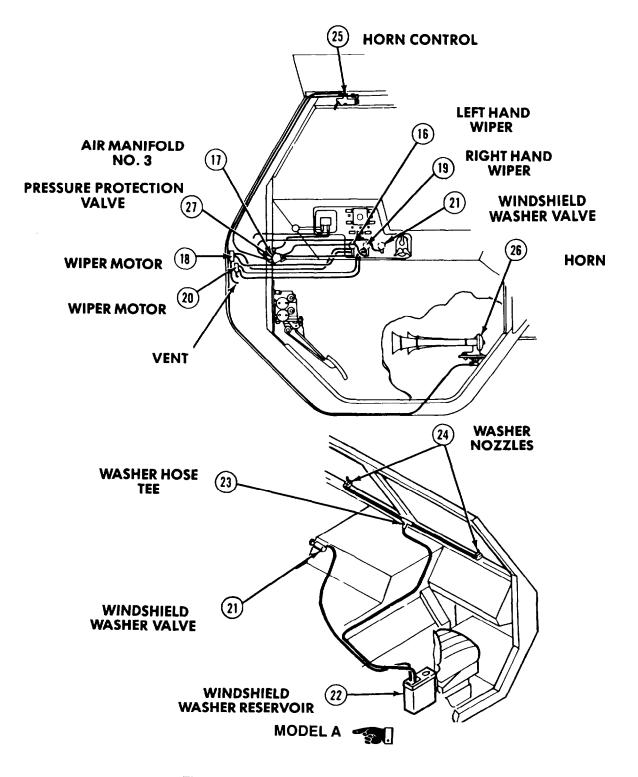
Figure 11-2. Wiper and Air Horn Hoses
