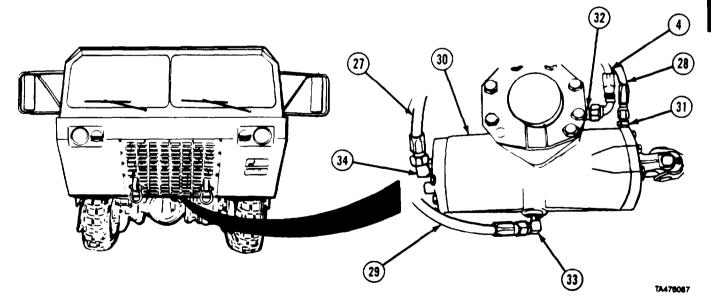
(10) Disconnect hoses (27, 28, 29 and 4) from steering gear (30).
