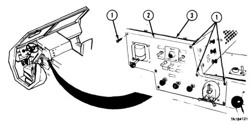
(1) Remove eight screws (1) and remove side panel (2) from console (3).
