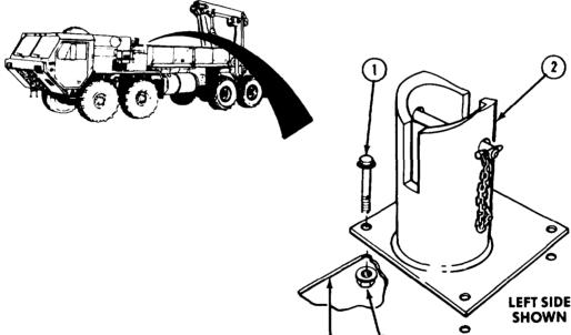
Both tow spade holders are removed and installed the same way.
