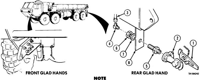
All glad hands are removed in the same manner except right front glad hand has straight nipple instead of 90 degree elbow. M984E1 front glad hands have 45-degree elbow on each glad hand.
