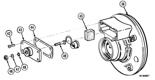
(21) Remove four screws (42), cover (43), gasket (44), and foam block (45) from end cover (36).
