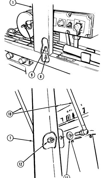
(4) Install two door pistons (10) on center panel (1) with two washers (11) and locknuts (12).
