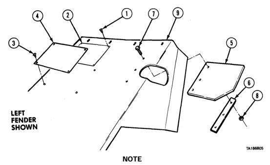
Data plates are installed the same way on left and right fenders.
