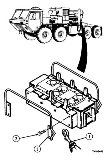
17-26. REMOTE CONTROL INTERCONNECT CABLE REMOVAL/INSTALLATION (M983). This task covers: c. Follow-on Maintenance a. Removal b. Installation **INITIAL SETUP** References Models None M983 with crane Equipment Condition Test Equipment None Condition Description TM or Para TM 9-2320-279-10 Shut off engine. Special Tools None Special Environmental Conditions None *Supplies* None General Safety Instructions None Personnel Required MOS 63S, Heavy wheel vehicle mechanic
