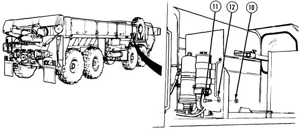
(3) Remove two nuts (10), screws (11), and grab handle (12).
