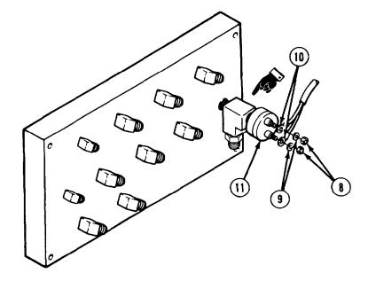
(3) Remove two nuts (8) and washers (9). Disconnect two electrical leads (10) from pressure switch (11).
