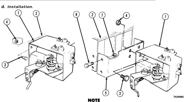
17-3. REAR CABLE TENSIONER REMOVAL/REPAIR/INSTALLATION (CONT).
