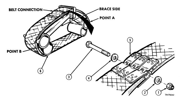
**a.** Disassembly. Remove locknut (1), washer (2), screw (3), washer (4), and belt (5) from tow adapter (6).
