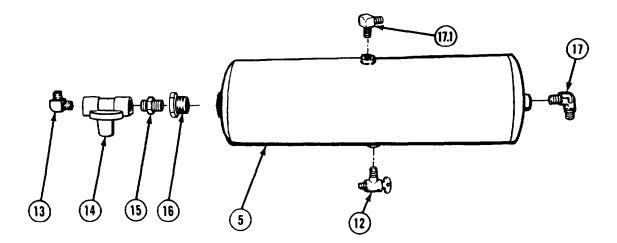
(6) Remove drain valve (12), elbow (13), pressure valve (14), nipple (15), reducer bushing (16), and elbows (17 and 17.1) from reservoir (5).
