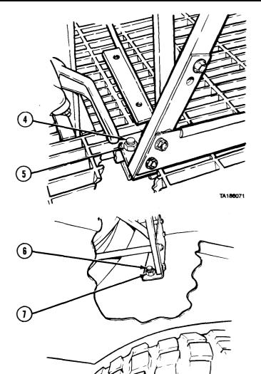
(4) Tighten two screws (6) and nuts (7).
