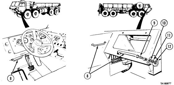
(3) Install grab handle (8) with two screws (9), washers (10), lockwashers (11), and nuts (12).
