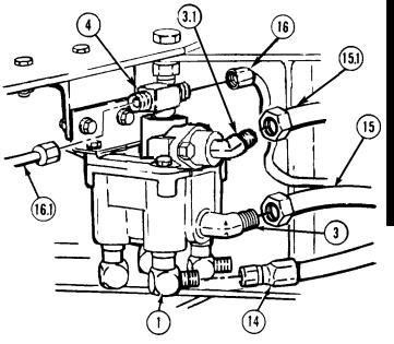
e. Left Rear Brake Relay Valve Removal.
