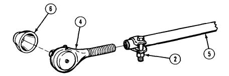
(2) Coat threads of tie rod end (4) with antiseize compound.
