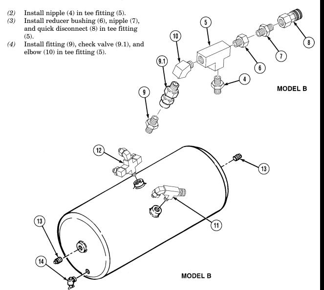
(5) Install tee assembly (11), cross assembly (12), two plugs (13), and drain valve (14).
