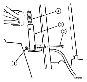
(1) Remove two nuts (1), screws (2), and support (3).
