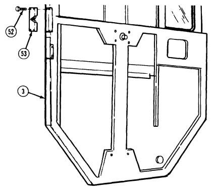
(36) Remove four screws (52) and female dovetail (53) from door (3).
