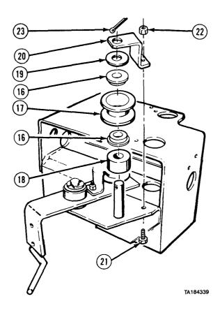
17-3. REAR CABLE TENSIONER REMOVAL/REPAIR/INSTALLATION (CONT).
