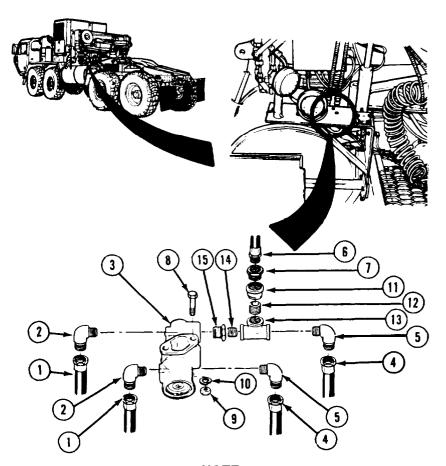
**NOTE** Tag and mark air lines before removal.
