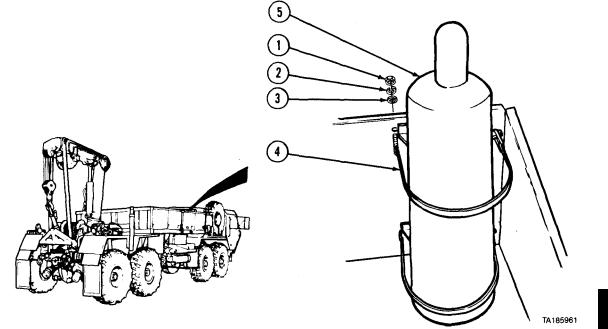
(1) Remove two nuts (1), lockwashers (2), washers (3), and two straps (4). (2) Remove acetylene bottle (5).
