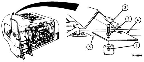
c. Top Access Panel Removal. Remove two locknuts (I), screws (2) washers (3), and top access panel (4) from pump module (5).
