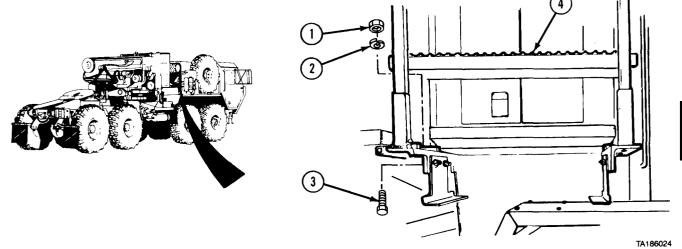
(1) Remove four nuts (l), lockwashers (2), and screws (3). (2) Remove right side catwalk (4).
