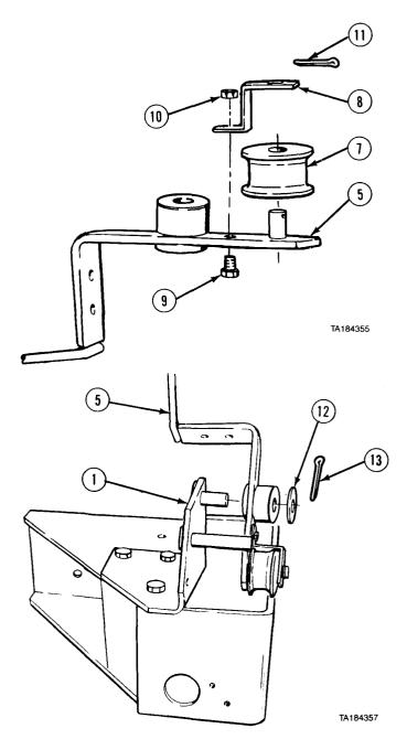
(5) Install pivot bracket (5) on bracket (1) with washer (12) and cotter pin (13).
