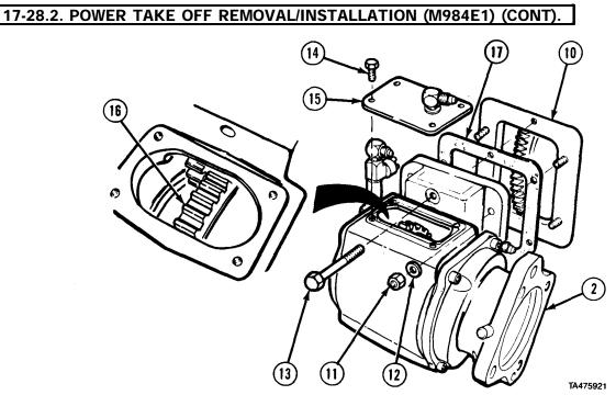
(9) Remove four screws (14) and cover plate (15) from PTO (2).
