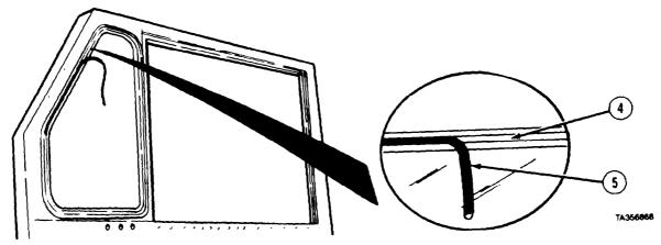
(6) Install locking strip (5) in center of locking channel (4).
