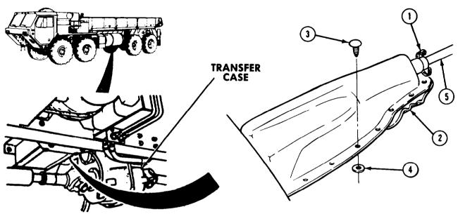
**NOTE** Boot is black plastic cover located on top right side of transfer case.
