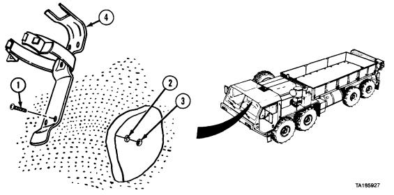
(1) Soldier A removes four screws (1) while Soldier B removes four lockwashers (2) and nuts (3). (2) Remove fire extinguisher mount (4).
