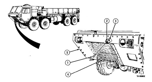
(1) Soldier A removes 16 screws (l), washers (2), and locknuts (3) while Soldier B holds skid plate grille (4) to skid plate (5).
