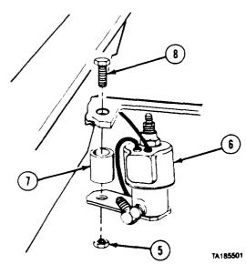
(4) Remove nut (5), screw (8), and solenoid assembly (6).
