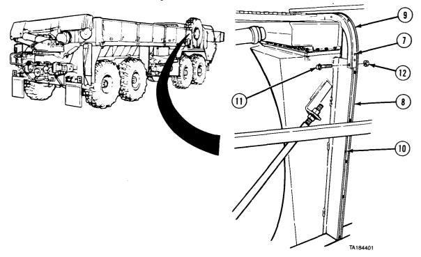
(3) Remove nine rivets (7) and rubber strip (8) from right side frame (9) and support (10).(4) Remove five screws (11), locknuts (12), and right side frame (9).
