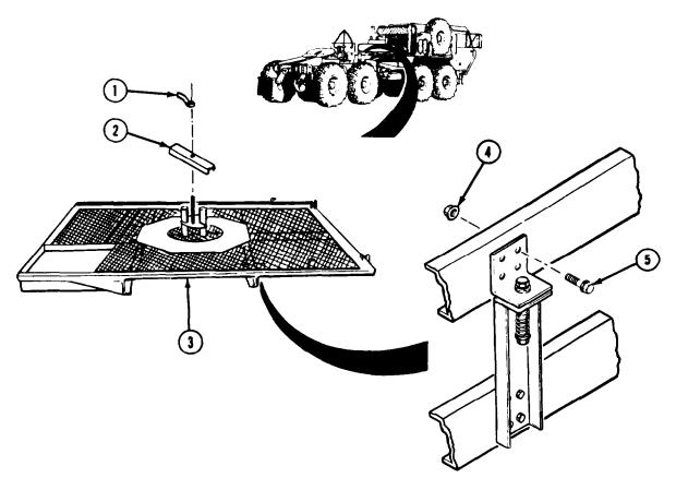
(1) Remove lever nut (1) and holddown plate (2).
