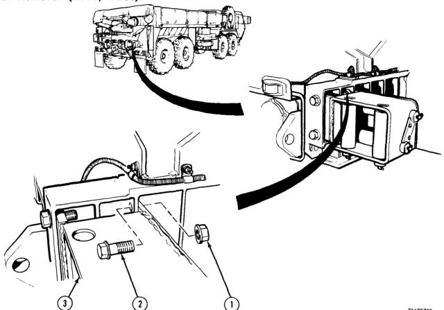
(1) Remove two nuts (1) and screws (2) from cable guide (3).
