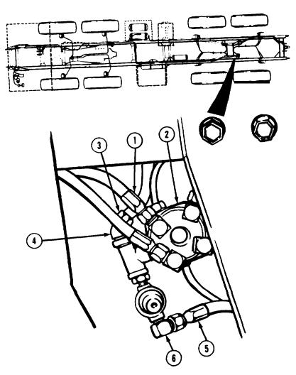
(4) Disconnect two control lines (7) from double check valve (8).
