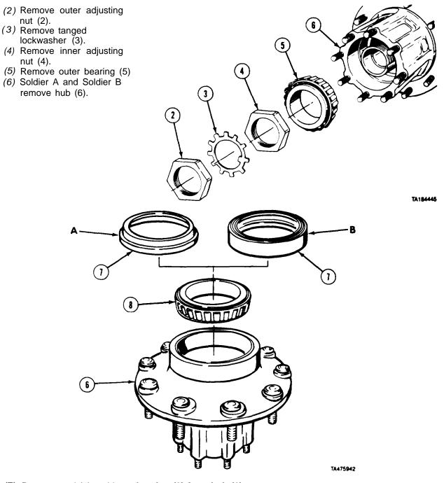
(7) Remove seal (7) and inner bearing (8) from hub (6).
