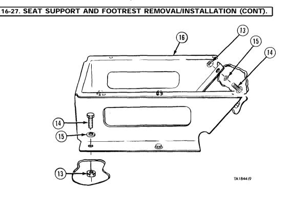
(5) Remove six nuts (13), screws (14), and washers (15). (6) Remove seat support (16).
