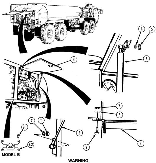
When door support rods are removed, door may slam shut and cause personal injury.
