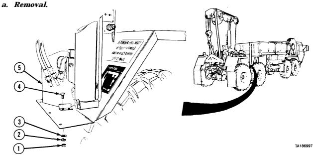
(1) Remove two nuts (1), lockwashers (2), washers (3), and screws (4) from outrigger beam (5).
