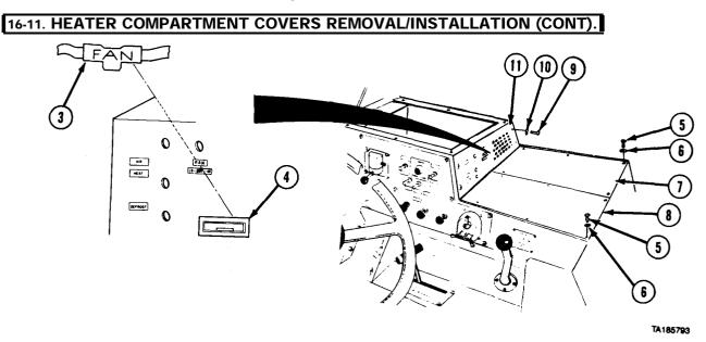
(2) Press tab at rear of each identification marker (3) and remove five identification markers,
