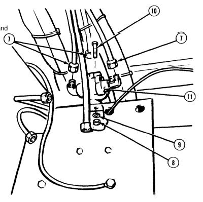
(5) Remove lower double check valve (5) and middle double check valve (6) from nipple (12).
