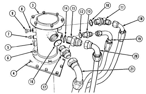
(2) Install filter housing (3) on reservoir (4) with four screws (5) and lockwashers (6). WARNING
