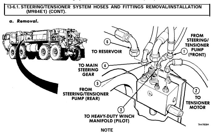
Position suitable container under vehicle to catch oil.Tag and mark hoses and fittings before removal.
